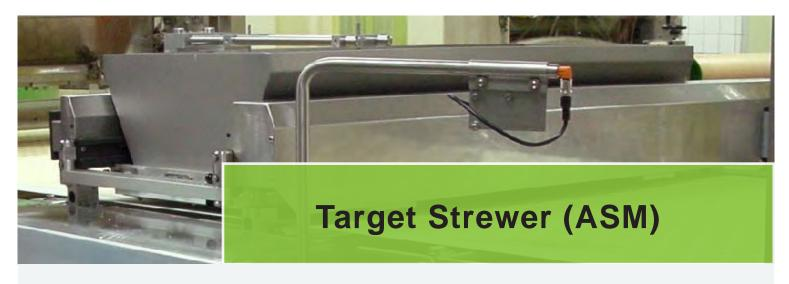
This machine is designed to place pre-selected amounts of strewing materials, directly on to the products on the oven conveyor.
