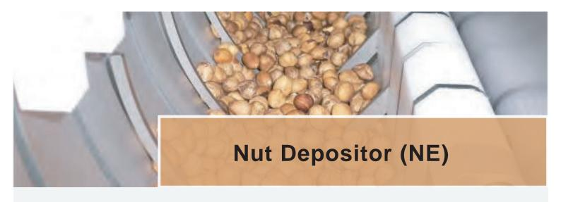
The Nut Depositor is designed to drop single calibrated nuts onto products with high efficiency and precision.
