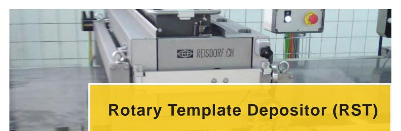
The Rotary Template depositor is designed and built for easy stenciling of soft doughs, pastes and aerated masses.
